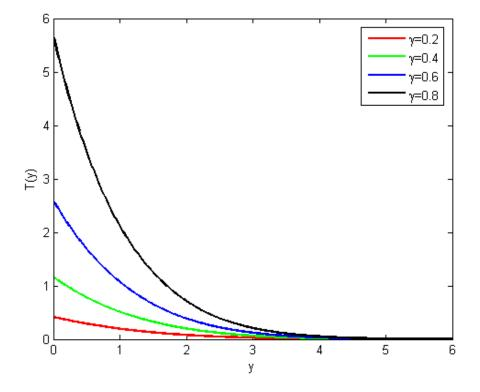
Fig.14: Temperature T against y for Pr=0.71, N=1, t=0.7.
