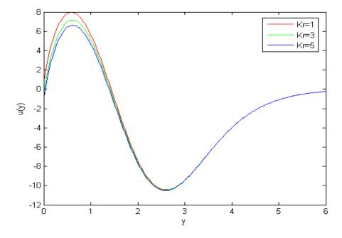
Fig.6: Velocity u against y for Gr=5, Gm=5, Pr=0.71, Sc=0.22, γ=0.5, N=1, α=0.5, t=0.7.
